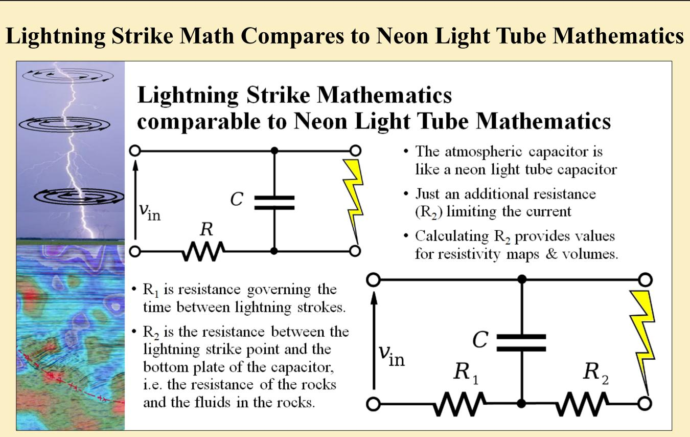
$R_2$  is apparent resistivity in the subsurface. Dynamic calculates this resistance at the surface, for apparent resistivity maps, and at depth, based on the Peak Current of the lightning strike. Hundreds to millions of these values are then interpolated to create apparent resistivity volumes, which have been shown to tie resistivity logs in a South Texas project. **1** Pending and **2** Issued U.S. Patents and **4** Prepared Submissions
