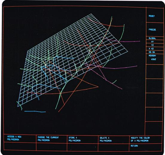
Seismic Data Analysis—The Picture System can be a powerful tool for interpreting seismic data. Here fault lines are displayed beneath a grid representative of the earth's surface. Color is used to identify lines belonging to a common fault plane.
