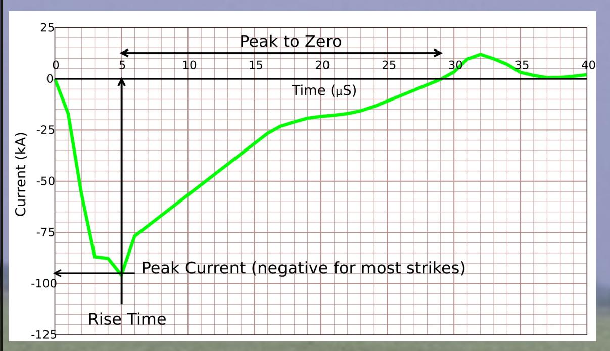
For data analysis, the recorded lightning data can be "cleaned" by omitting strikes with excessively arge semi-major axis, by omitting strikes with obviously erroneous values (such as a Rise Time of 0.0  $\mu$ S), and by omitting strikes detected by nly two sensors. Many strikes of doubtful accuracy are eliminated by more than one of these
