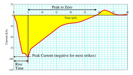
16. Peak current is the maximum value of current measured for the lightning strike. Measured values range from about -300 kA to +450 kA, but most are between -50 kA and -5 kA. Lightning strikes with the absolute value of peak current less than 5 kA are rarely recorded.
