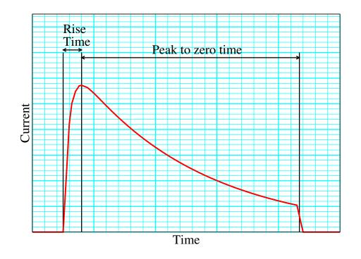
63. That general appearance suggested an analog to lightning. This is the waveform of the voltage across a neon tube in a simple circuit.
