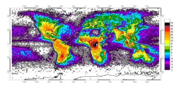
3. Lightning strikes are recorded by the National Lightning Detection Network (U.S.) and Global Lightning Dataset GLD360 (worldwide). These networks are owned and operated by Vaisala, a company based in Helsinki, Finland, which also makes the sensors. Many other countries have lightning detection networks often owned by national governments. Vaisala has supplied or installed lightning detection networks in 45 countries.
