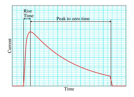
80. Look at this plot, courtesy of the U.S.. It is the typical time domain IP waveform. A very similar shape. Apparent permittivity can be calculated from either the rising curve or the falling curve. We cannot use the falling curve, because our input is not a square wave. But we do have a nearly vertical onset, so we can calculate something which we can call apparent permittivity from the rise time.
